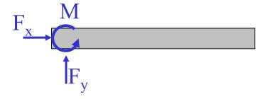
The magnitude and direction of the forces and couple provided by the support depend on the loads applied to the member.
