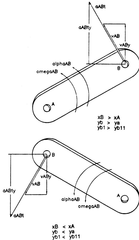
Fig. 3. The signs associated with angular velocity/acceleration of the links AB and BC are determined by comparing values of the appropriate co-ordinates of the kinematic polygons. Anti-clockwise rotation or acceleration is positive, so if one, and only one, of the pair of conditions below is untrue, then the rotational velocity/acceleration is negative (clockwise).
