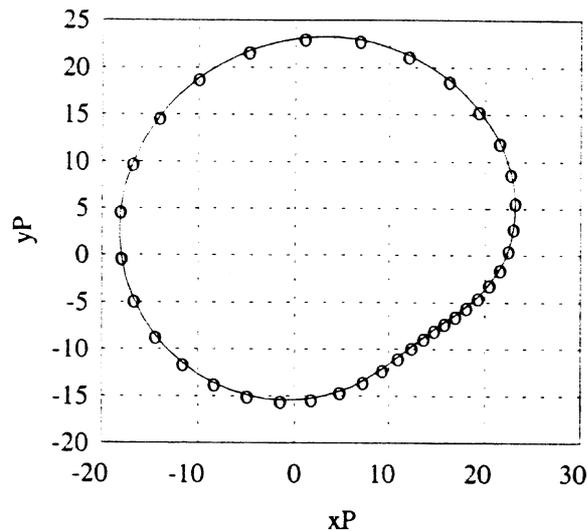
Fig. 7. Pathline for point P on the extended coupler rod, ABP;  $AP = AB * 4$ .
