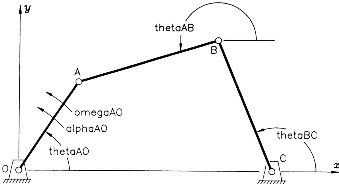
Fig. 1. Fourbar linkage, open configuration. The model is solved for nondimensional data as presented in Norton [1], Table P7-1, row c, p261:  $AO = 10$ ,  $AB = 6$ ,  $BC = 8$ ,  $OC = 3$ , crossed,  $\theta_{AO} = 45^\circ$ ,  $\omega_{AO} = -15$ ,  $\alpha_{AO} = -10$ .
