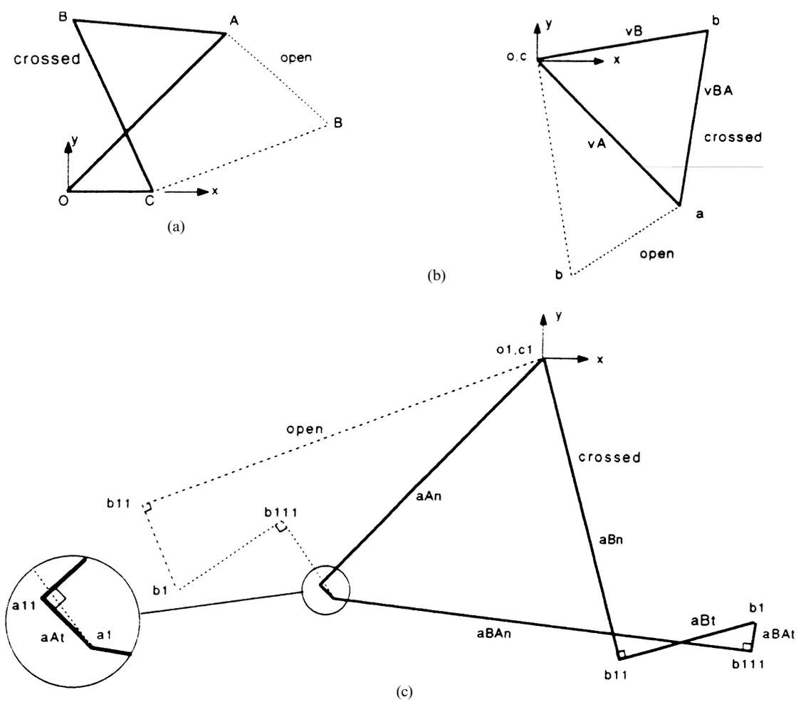
Fig. 2. Co-ordinate generation. Input co-ordinates (twelve) appear with asterisks. (a) Position diagram, crossed and open. Upper case letters denote the ends of links. (b) Velocity diagram, crossed and open. Lower case letters denote the ends of velocity vectors. (c) Acceleration diagram, crossed and open. Lower case letter with single, double, or triple numerals denote the ends of acceleration vectors.
