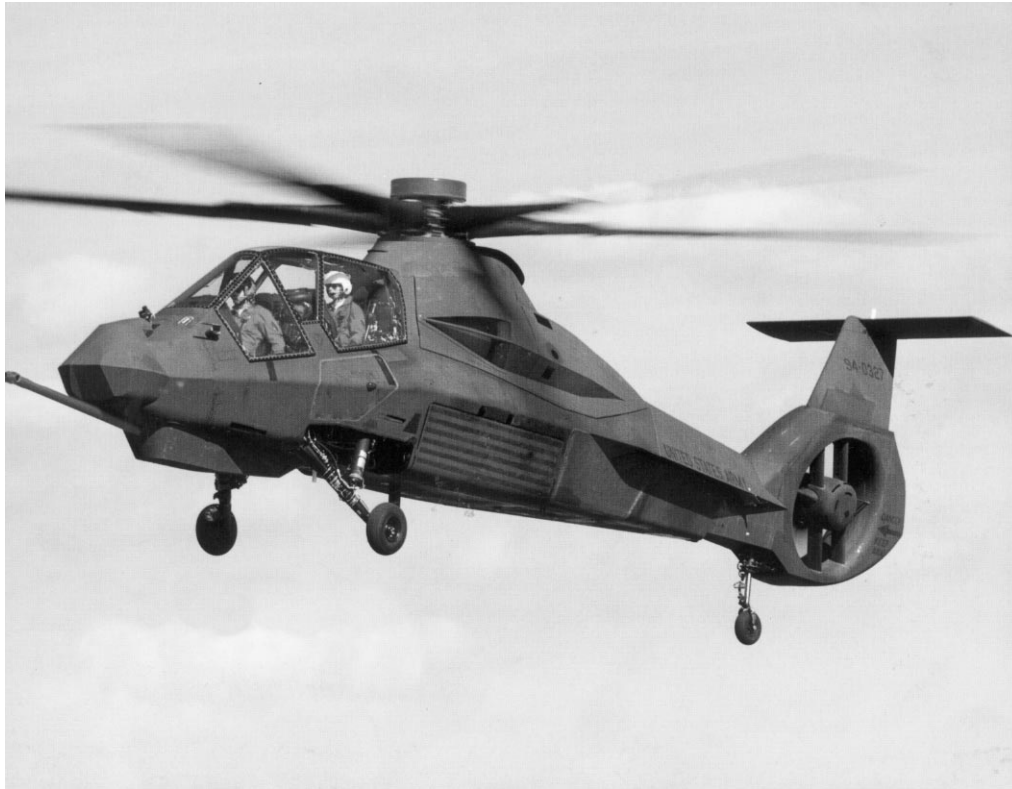
Fig. 1. The Comanche helicopter under development by the Boeing-Sikorsky team incorporates an advanced bearingless rotor system that increases reliability by replacing pitch bearings, lag hinges, and flap hinges used in conventional articulated rotor systems with a flexbeam/torque tube arrangement. Courtesy: Sikorsky Aircraft.
