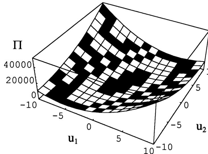
Fig. 10. The  $\Pi$  functional for equilibrium displayed in 3-D with Mathematica code.
