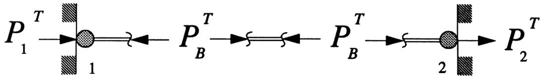
Fig. 7. Free-body diagram of bar between rigid walls in compression under increase in temperature. Nodes shown shaded.
