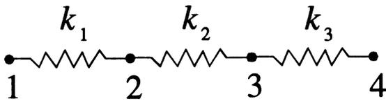
Fig. 5. Four-node, three-element chain-like structure.
