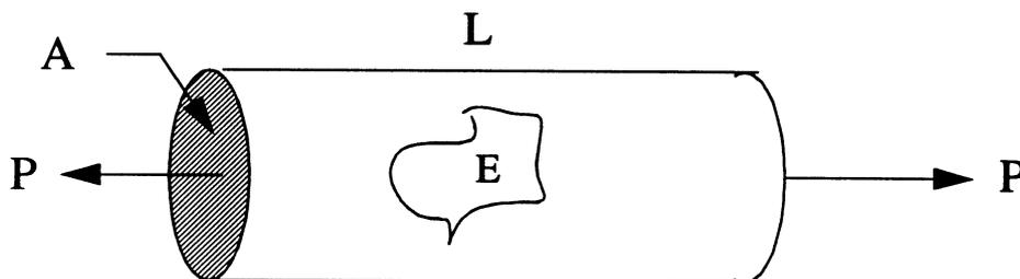
Fig. 1. Bar with elastic modulus  $E$ , length  $L$  and section area  $A$  under tensile force  $P$ .
