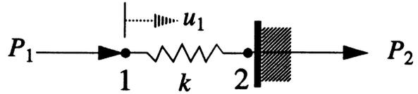
Fig. 4. Bar element under the influence of  $u_1$  with  $u_2$  fixed.
