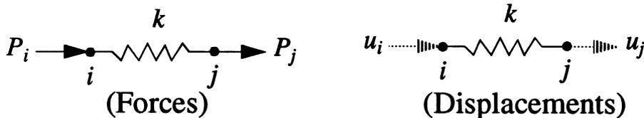
Fig. 3. Bar element showing nodal forces and nodal displacements.
