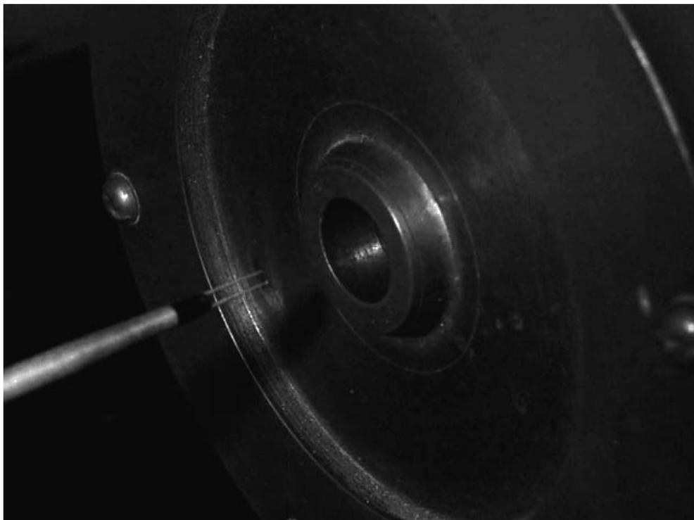
Fig. 7. Hot wire probe in calibration rig.
