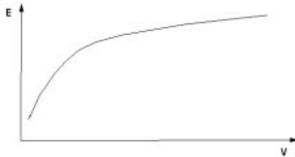
Fig. 5. Hot wire calibration curve.
