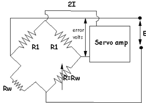
Fig. 4. Hot wire bridge circuit.
