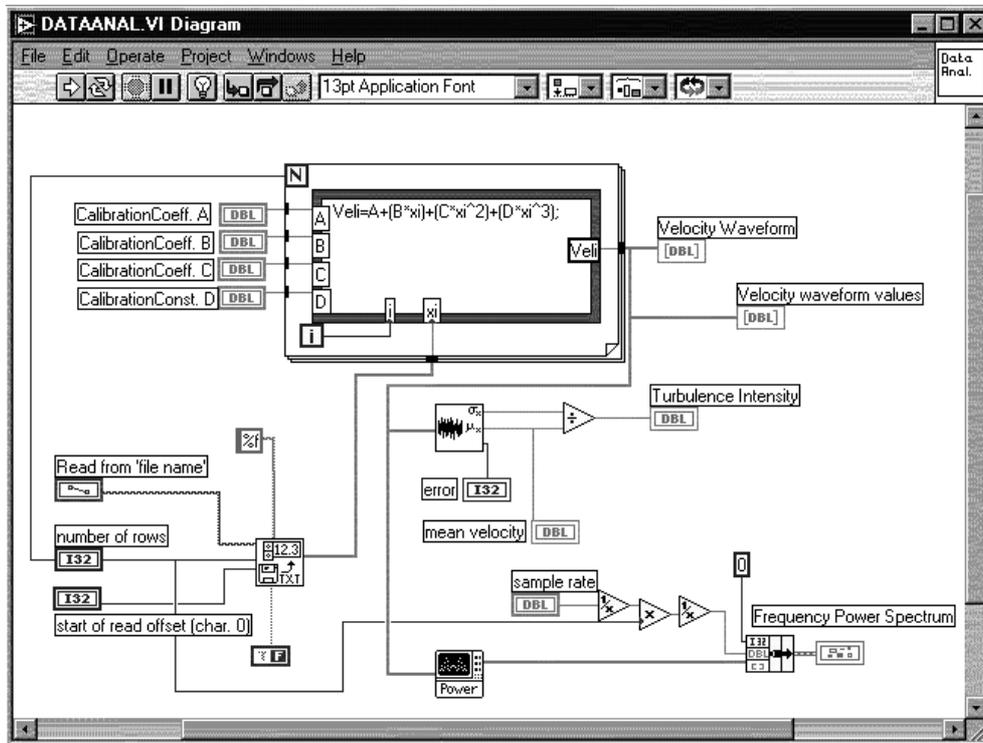
Fig. 9. Diagram of hot wire anemometry analysis.
