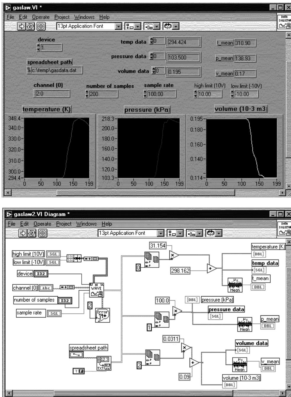
Fig. 2. (a) Front panel of PVT experiment VI; (b) Diagram of PVT experiment VI.
