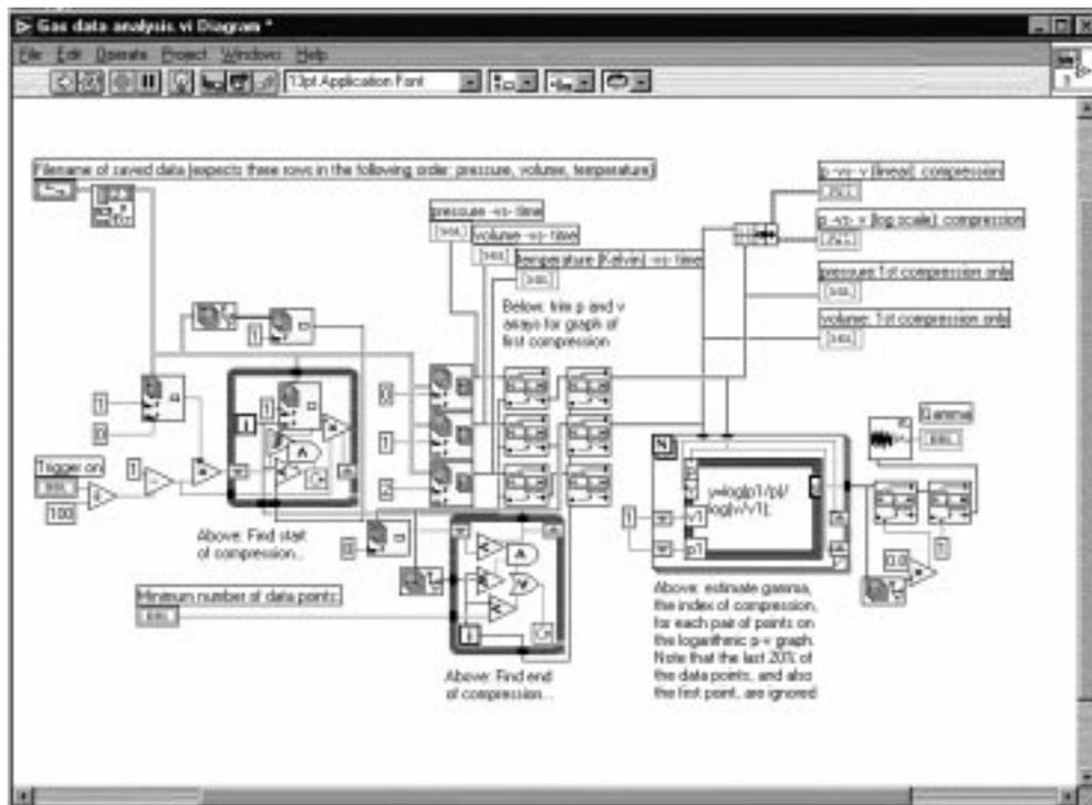
Fig. 3. Diagram of PVT extended analysis VI.
