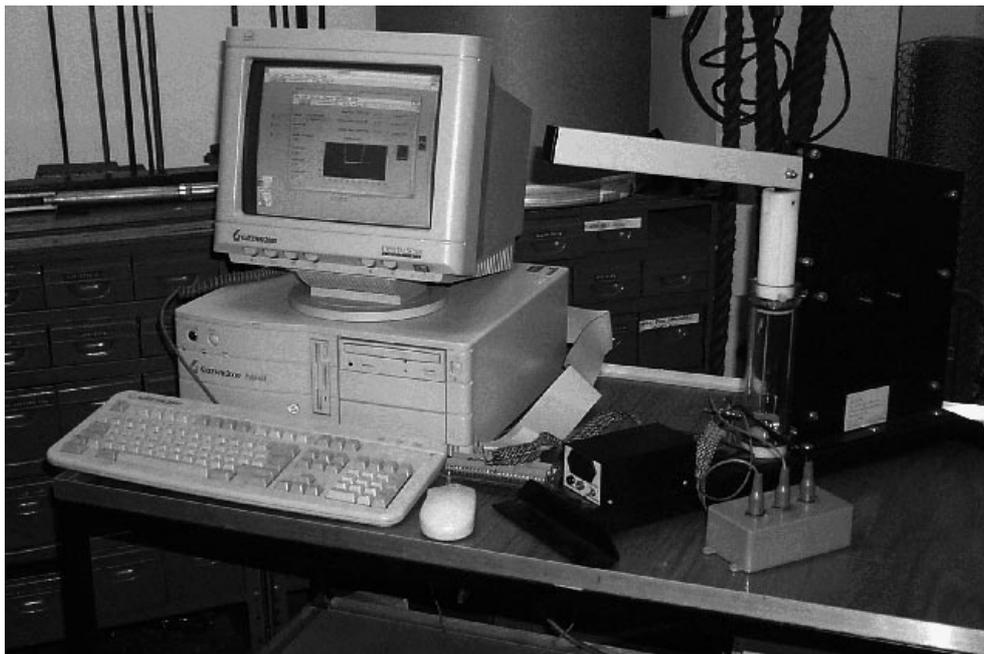
Fig. 1. PVT gas law rig with data acquisition workstation.
