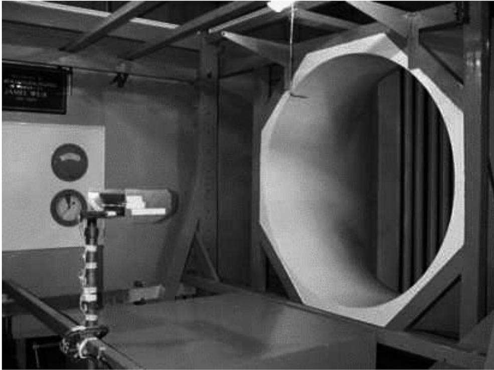
Fig. 10. University of Strathclyde wind tunnel showing a sting mounted model.
