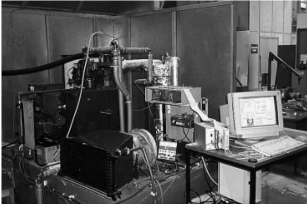
Fig. 11. CHP rig with LabVIEW workstation and SCXI chassis.
