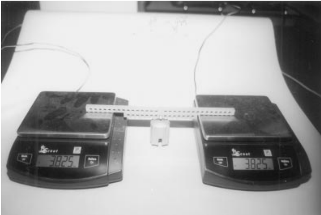
Fig. 1. Our apparatus for demonstrating the normal force of a bridge abutment.
