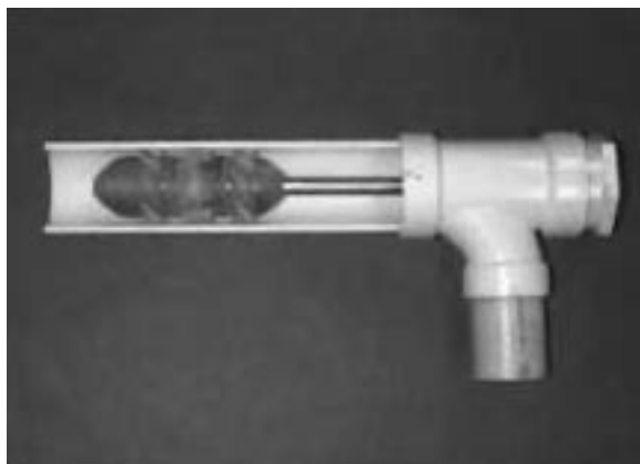
Fig. 7. Cross-section of Spring 1996 two-stage axial flow pump.
