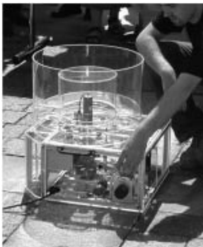
Fig. 14. Mechatronic product to shoot and train with uni-hockey balls.
