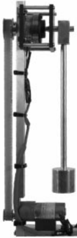
Fig. 3. SPENDULAP initial positioning mechanism, consisting of lift motors, gears, pulley, clutch, and brake (brake not shown).
