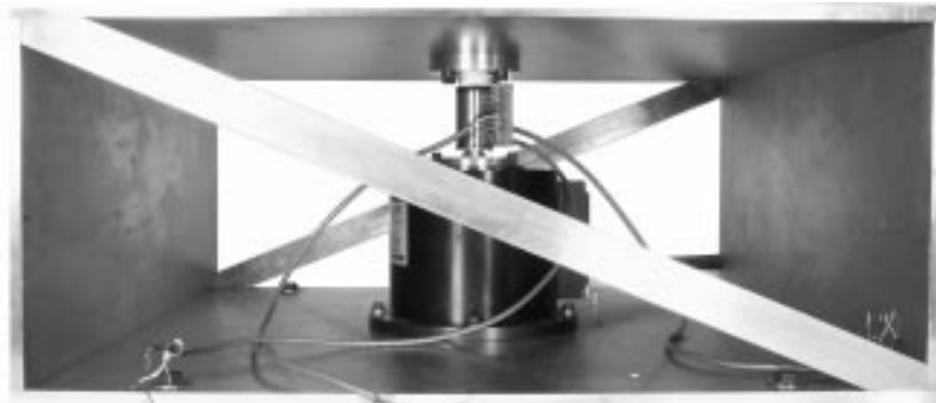
Fig. 4. Brushless direct-drive DC motor and slipping.
