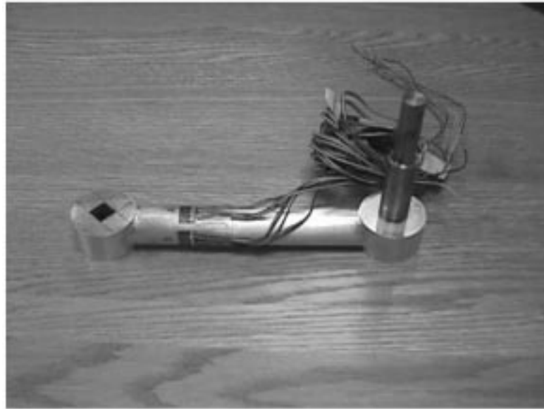
Fig. 4. Prototype crank arm with strain gage rosettes.
