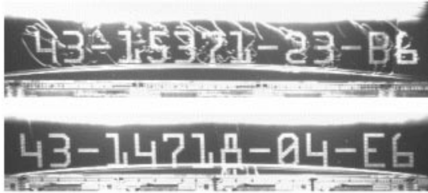
Fig. 2. Wafers with damaged characters.
