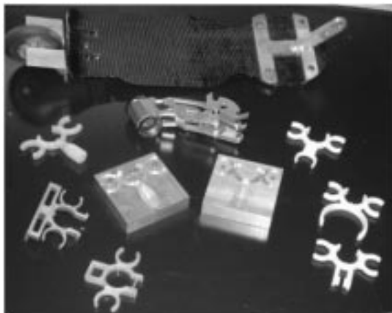
Fig. 1. Sample results of scooter project: clip mold, sample clips, re-engineered steering and hinge assembly, and composite scooter base.
