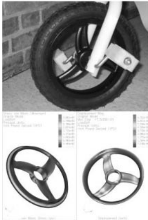
Fig. 10. Tricycle rim design for tubular tires and structural analysis results.
