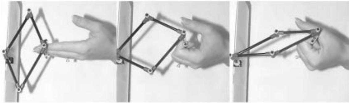
Fig. 4. Prototype of the hand rehabilitation robot demonstrating the range of motion of the five-bar mechanism.
