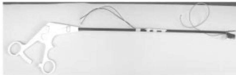
Fig. 1. A surgical grasping instrument with PZT sensors attached to the shaft and grippers.
