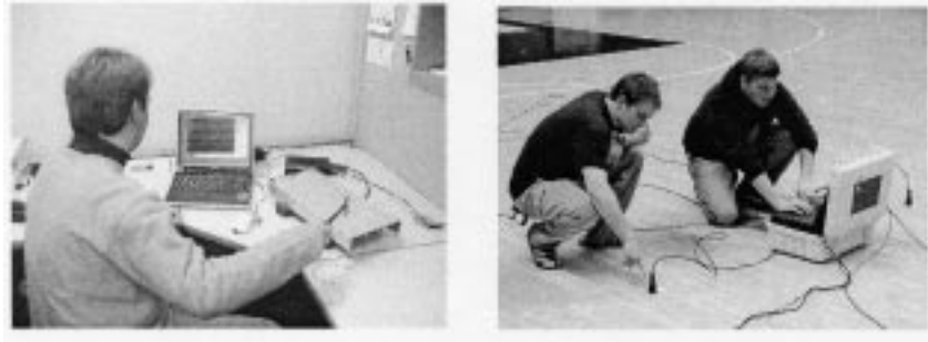
Fig. 2. Two student experimental set-ups showing an inexpensive, custom-built data acquisition system (left) and a battery-powered portable data acquisition system (right).
