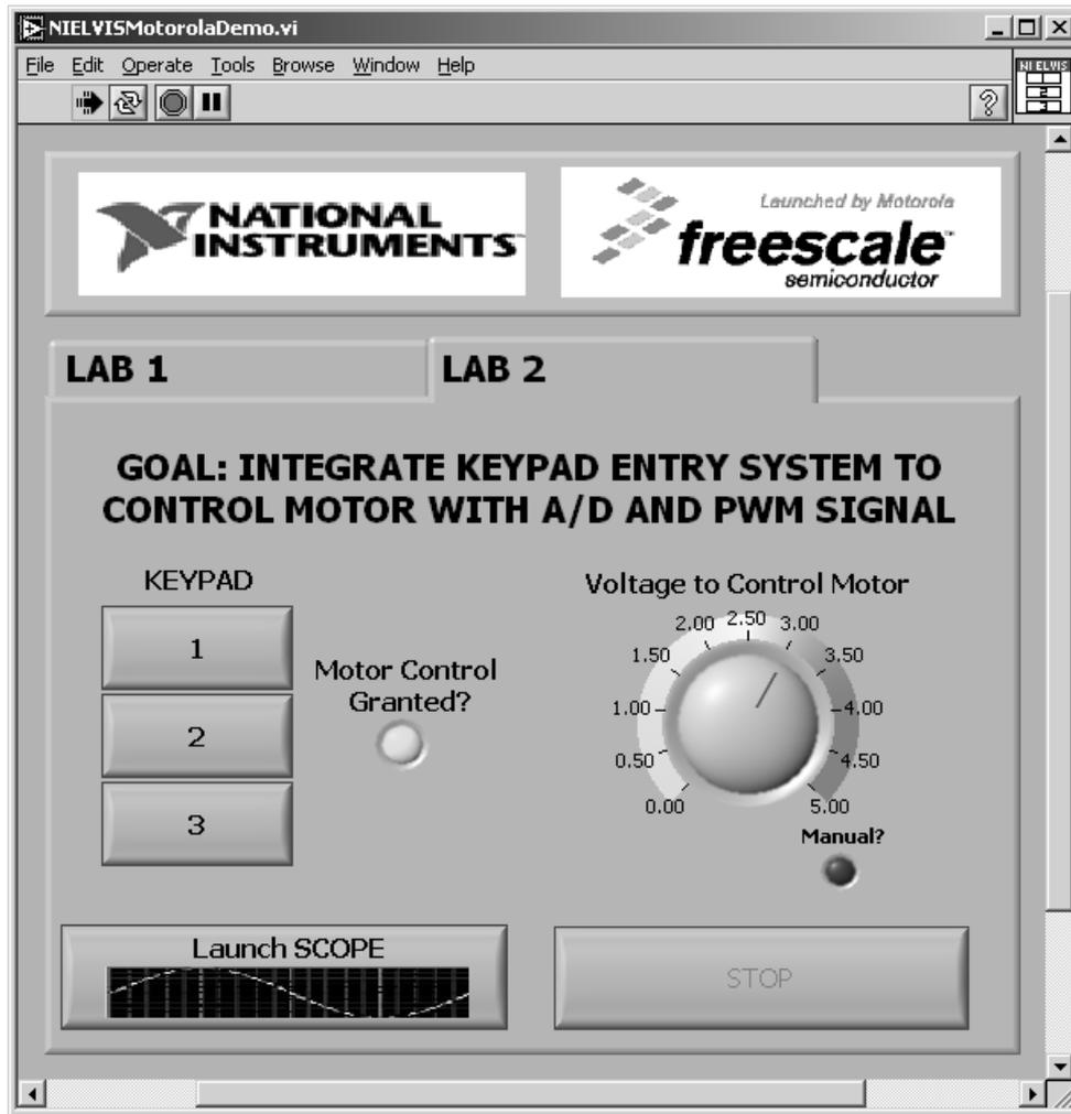
Fig. 2. Motor control front panel.
