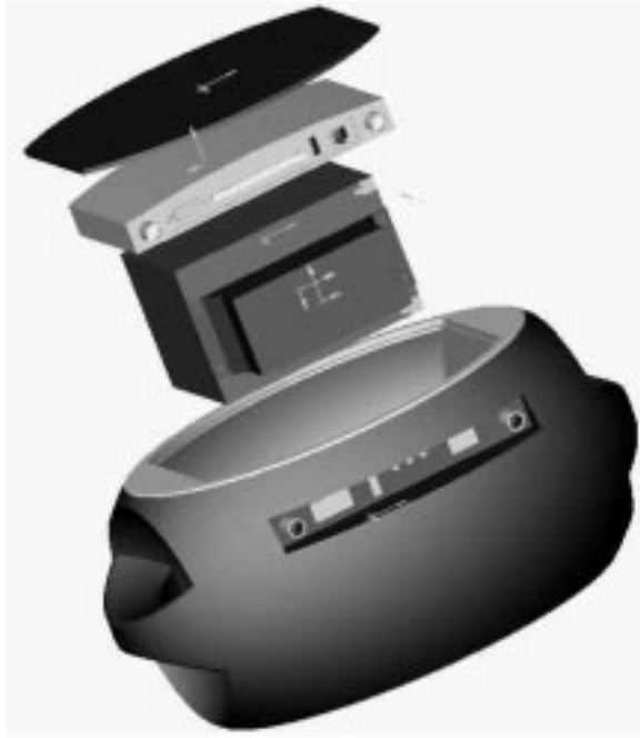
Fig. 2. Portable, solar-powered wireless communication access point.
