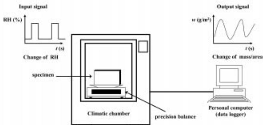
Fig. 2. Sketch of experimental set-up.
