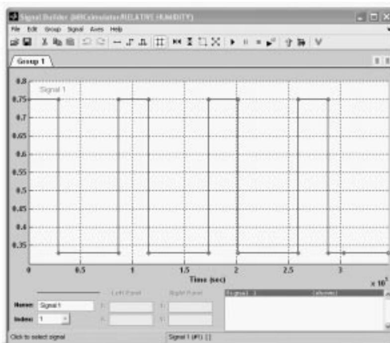
Fig. 3. Cycles of relative humidity variation inside the climate chamber.
