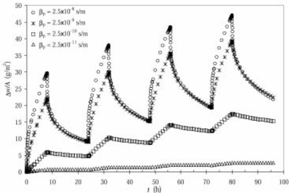
Fig. 6. Numerical analysis of the influence of varnish layers over a spruce specimen.
