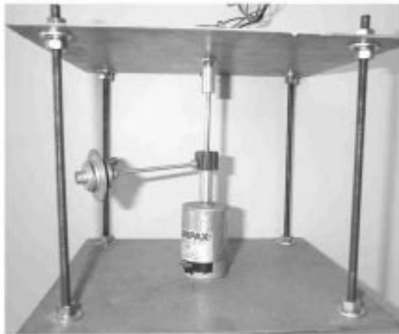
Fig. 3. Single link robot mechanical system with top support plate.
