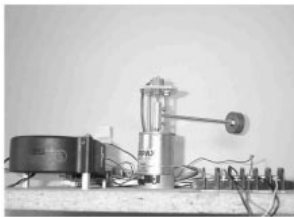
Fig. 4. Single link robot mechanical system with axial mount.
