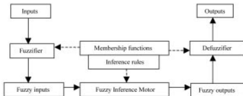
Fig. 9. Scheme of a typical fuzzy controller.
