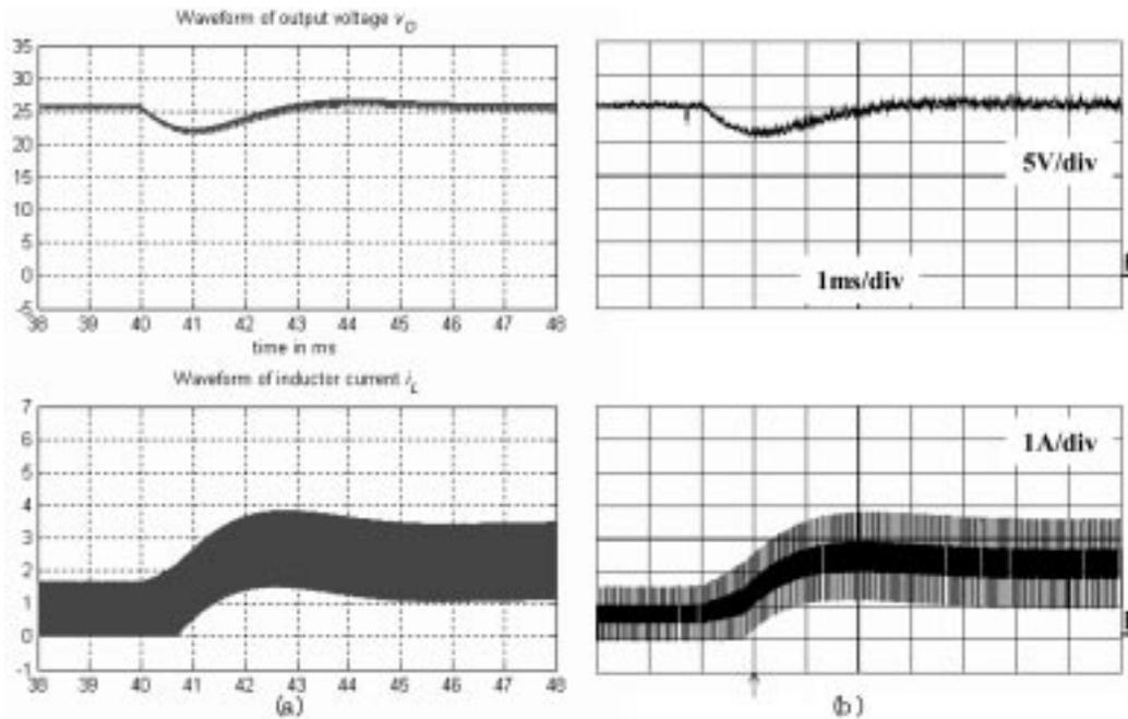
Fig. 14. The (a) simulation and (b) experimental results of the load change transient responses of the boost converter circuit in Fig. 11.
