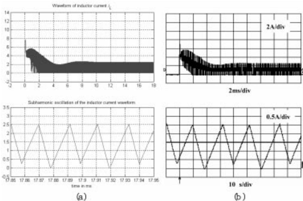
Fig. 10. Sub-harmonic oscillation phenomenon in the (a) simulation and (b) experimental start-up inductor current responses of the switching converter circuit in Fig. 6.
