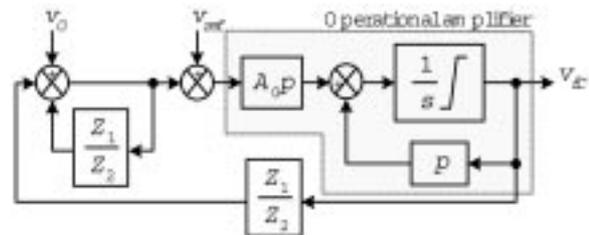
Fig. 3. The signal flow block diagram equivalent to the feedback controller in Fig. 1.
