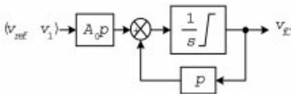
Fig. 2. A Simulink behavior model that implements the open loop transfer function in Equation (3) of an OPA.
