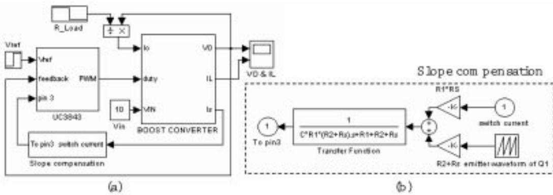
Fig. 12. The (a) Simulink behavior model of the experimental circuit in Fig. 11; (b) the behavior model of the slope compensation circuit.
