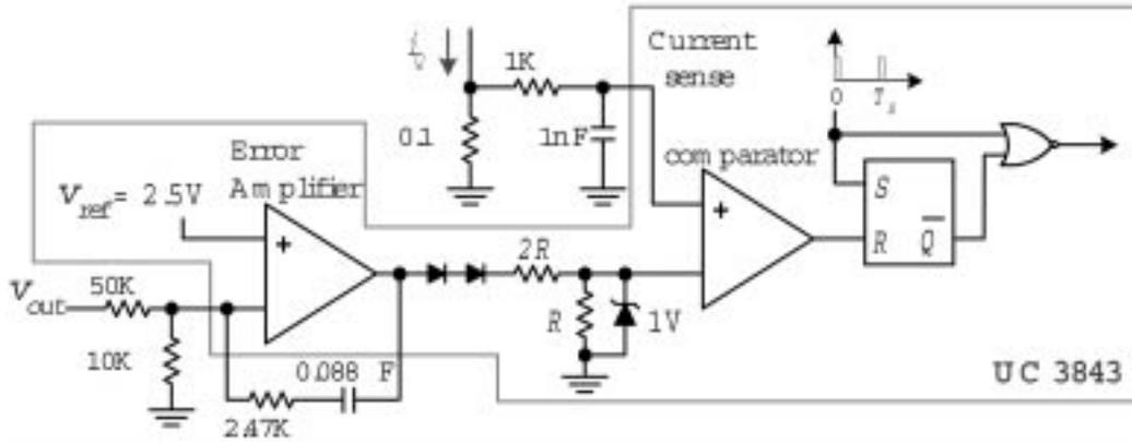
Fig. 7. The control circuit diagram to drive the power transistor in Fig. 6.
