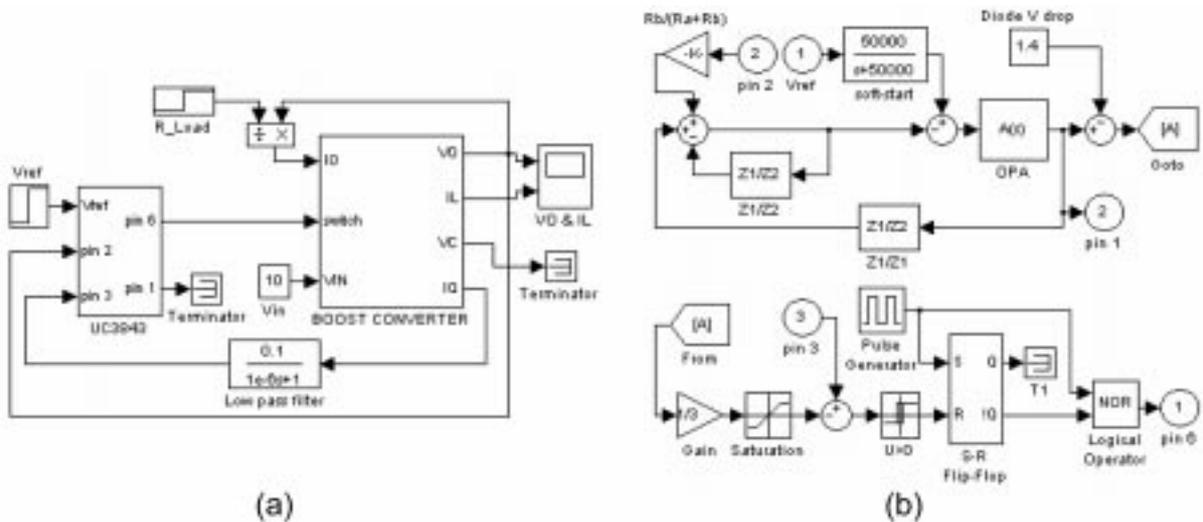
Fig. 8. (a) The Simulink behavior model of the experimental circuit in Fig. 6; (b) the behavior model of the PWM control IC UC3843.
