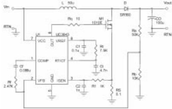
Fig. 6. A boost-type experimental switching converter circuit using UC3843 without slope compensation.
