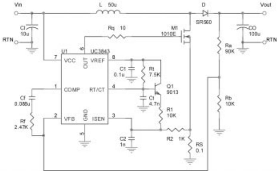
Fig. 11. A boost-type experimental switching converter circuit using UC3843 with slope compensation.
