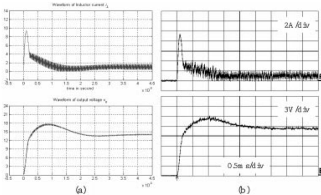
Fig. 9. The (a) simulation and (b) experimental start-up transient responses of the DC–DC switching converter circuit in Fig. 6.
