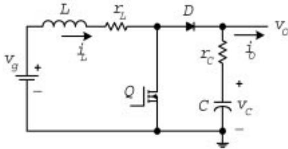
Fig. 4. The boost-type switching converter circuit.
