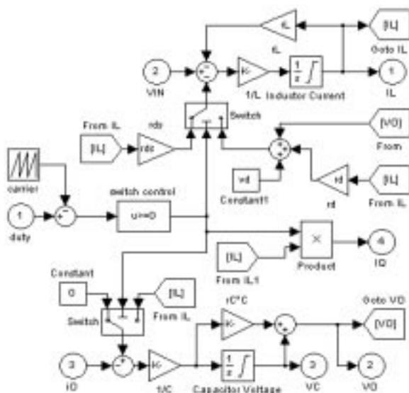
Fig. 5. The Simulink behavior model of a boost-type switching converter circuit with parasitic parameters and power switch current output.
