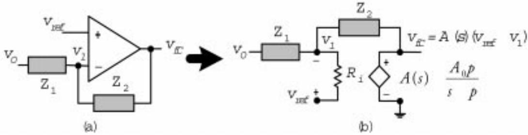
Fig. 1. (a) A general form of feedback controller implemented by using an OPA; (b) its equivalent circuit.
