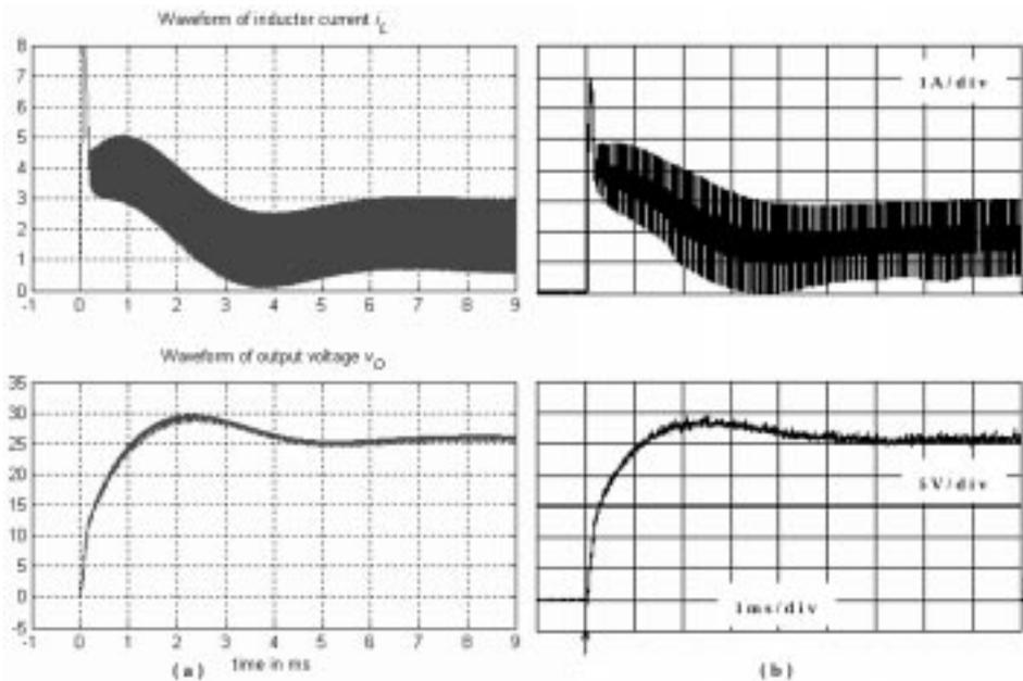
Fig. 13. The (a) simulation and (b) experimental start-up transients of the boost converter circuit in Fig. 11.
