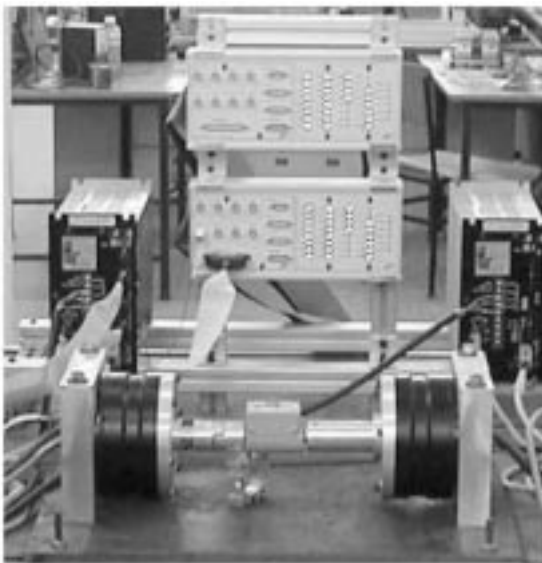
Fig. 1. The HILS test stand.
