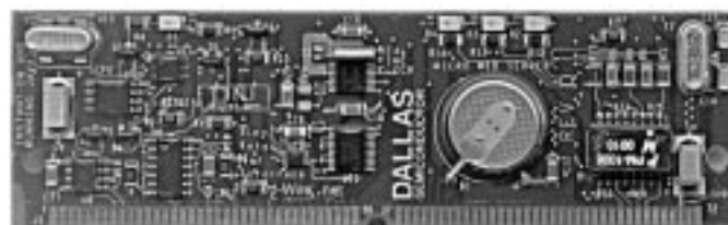
Fig. 3. TINI board without casing used as a node within the experimental network [13].
