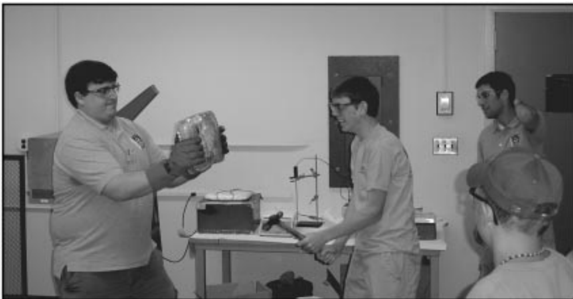
Fig. 3. Instructor Matt Perricone holds an ice and newspaper composite, while student Joseph Barron prepares to take a swing with a hammer to demonstrate the composite strength.
