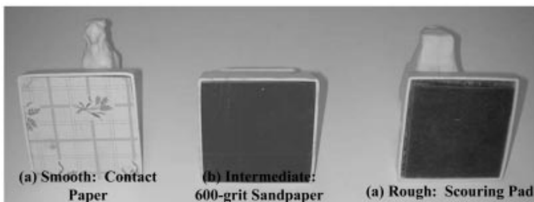
Fig. 3. Objects placed in order of increasing roughness: (a) contact paper, (b) 600-grit sandpaper, and (c) scouring pad.
