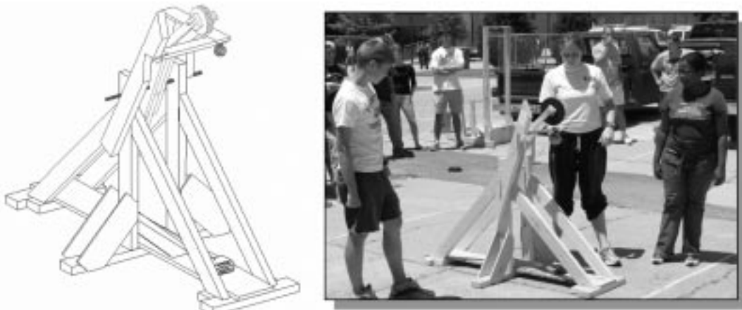
Fig. 1. AutoCAD ® rendering of a BE1250 freshman team-designed catapult (left) and photograph of the team testing their constructed catapult during the departmental competition (right).
