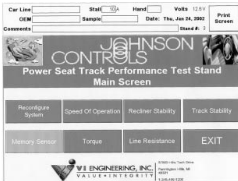
Fig. 10. Virtual instrument for controlling a seat power track stability test stand. Courtesy of Johnson Controls, Detroit, MI.
