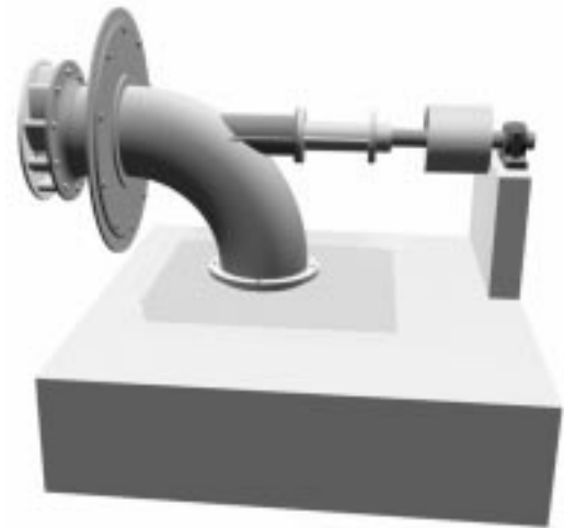
Fig. 4. Solid model of centripetal turbine.
