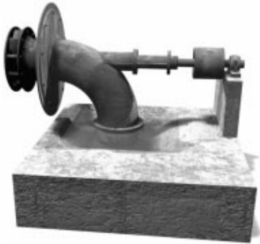
Fig. 6. Final model of centripetal turbine.
