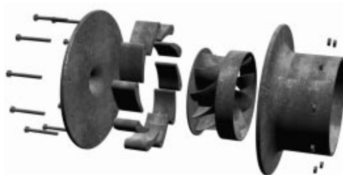
Fig. 8. Exploded view of centripetal turbine.
