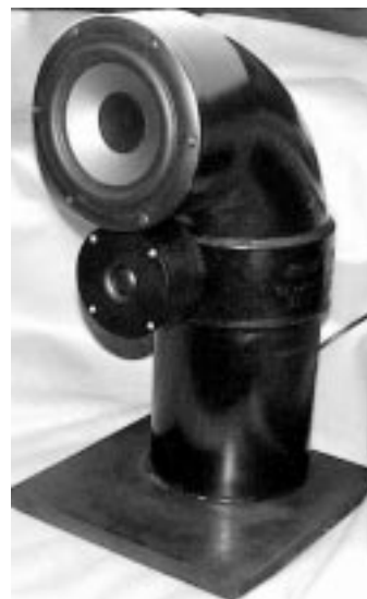
Fig. 7. Loudspeaker design using PVC and MDF.
