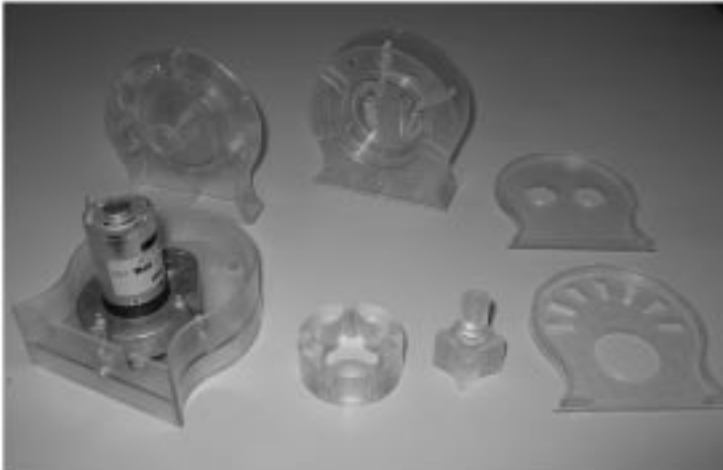
Fig. 5. Prototypes obtained by stereo lithography for size verification.
