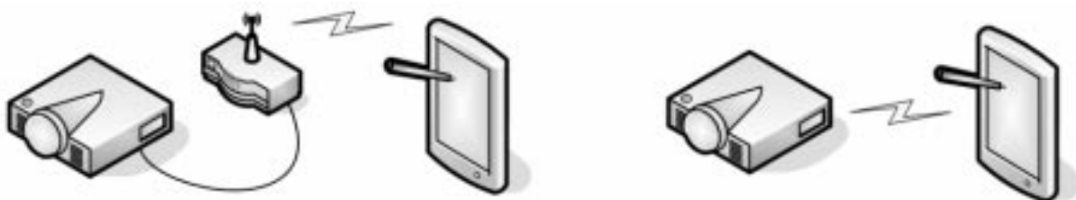
Fig. 1. Wireless connection alternatives: indirectly through an multimedia access point (left) or directly with a wireless projector (right)
