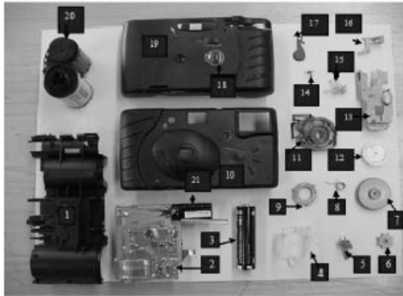
Fig. 2. Keeping track of product dissection of a camera using edited photographs. 1. Inner Housing and Aperture; 2. Flash and Printed Circuit Board; 3. Battery (1.5V AA); 4. Viewfinder; 5. Exposure Remaining Advance; 6. Film Advance Bracket; 7. Thumb Wheel; 8. Spring; 9. Ring Adapter; 10. Front Housing; 11. Lens Housing; 12. Exposure Remaining Wheel; 13. Shutter Button and Support; 14. Shutter Spring; 15. Interposer; 16. Shutter Activator; 17. Shutter; 18. Lens; 19. Rear Housing; 20. Film (35 mm Film 27 Exposures); 21. 120 MicroFarad Capacitor.
