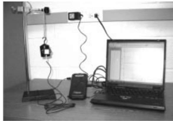
Fig. 3. Damped vibrations experiment: Mass-spring (rubber band) system with accelerometer
