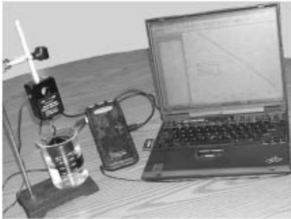
Fig. 1. Buoyancy experiment: a mass, suspended on a force sensor, is placed in a liquid to examine Archimedes Principle
