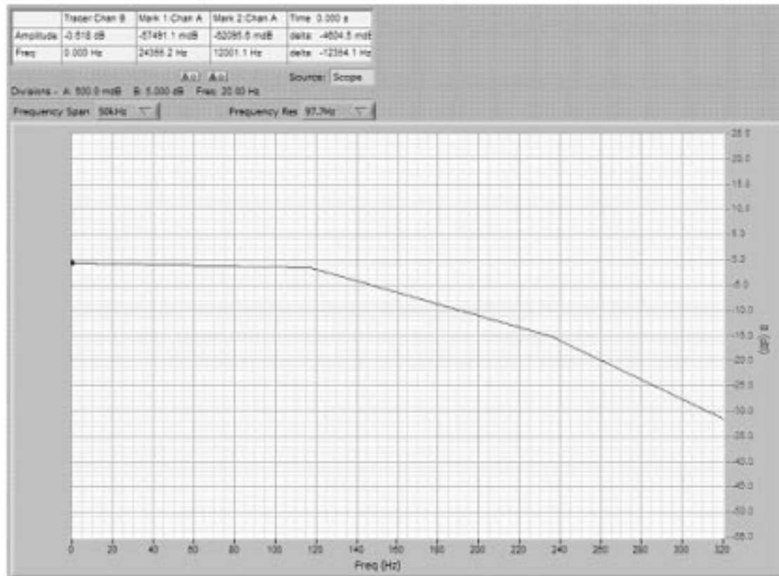
Fig. 10. Filter frequency response
