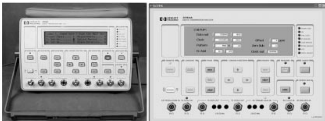
Fig. 7. The digital transmission analyzer HP 3784A (left), and its VI panel (right).
