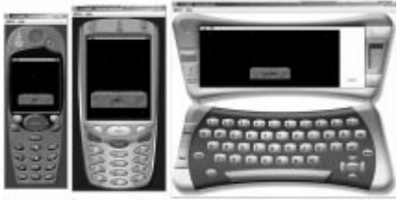
Fig. 2. Sun mobile phone emulators. From left to right we have MediaColorSkin (177×180), DefaultColorPhone (289×240) and QwertyDevice (204×540). Each emulator uses different screen sizes.
