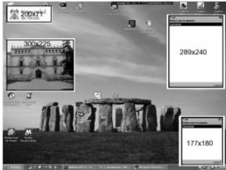
Fig. 1. Desktop computer screen with 1280 \times 1024 pixels resolution and four images overprinted: one little logo ( 200 \times 71 ), one small photograph ( 300 \times 225 ) and two screen captures show the typical resolution of Sun mobile phone emulators.
