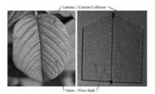
Fig. 1. Fuel cell bipolar plate design generated from an analogy to a leaf.
