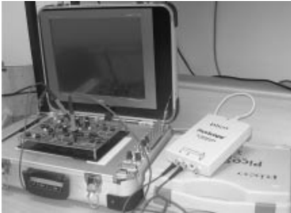
Fig. 10. Virtual measurement system used for chaos training boards experiments.
