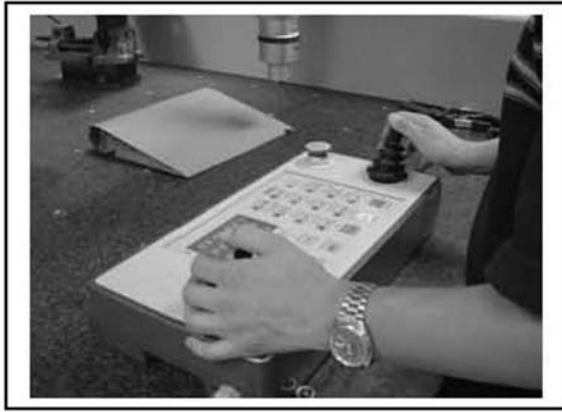
Fig. 5. Coordinate Machine Measurement (CMM) of one of the aircraft's components.
