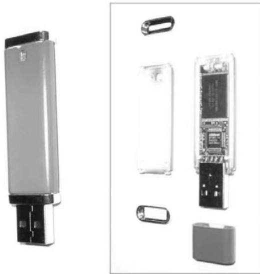
Fig. 5. 128MB USB flash memory drive before disassembly—left, disassembled—right. Overall dimensions approx. 2.5 \times 0.75 \times 0.375 inches.
