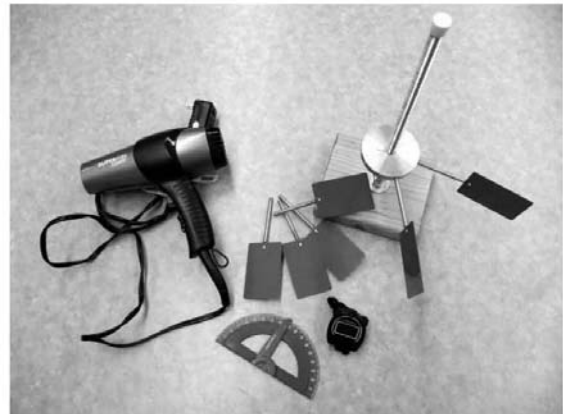
Fig. 5. Hardware for the wind turbine activity in the Wind and Water Power Kit.
