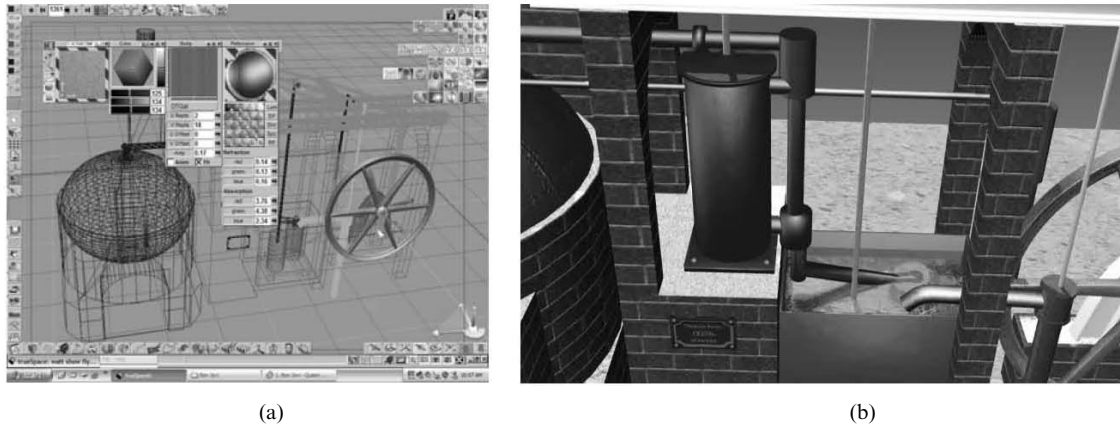
Fig. 5. 3D animated model of Watt's steam engine: a—the wire-frame for the graphics, designed according to the original drawings; b—a screenshot of the final product (Courtesy Radu Sporea).
