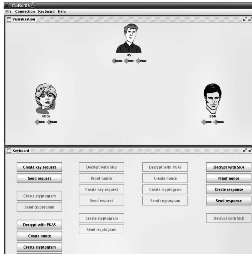
Fig. 1. Screenshot portion of the CoBo software displayed after the Needham-Schroeder Protocol and the "Alice" role have been selected.
