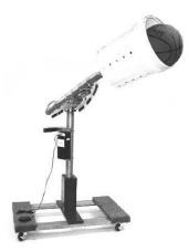
Fig. 5. Switch activated ball thrower [41].
