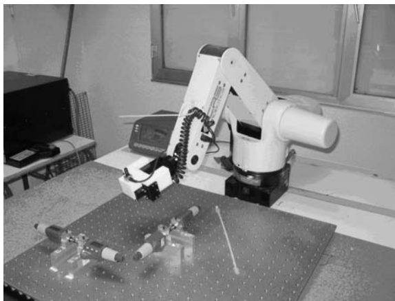
Fig. 5. Robot arm, digital viewer and micrometers in supports for the module tests.
