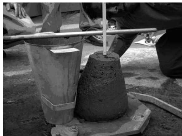
Fig. 2. Contractor performing ASTM C143 slump test.
