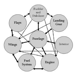
Fig. 1. Mechanical sub-systems and their inter-dependencies for a small Cessna type airplane. Only geometrical and structural inter-dependencies are shown.
