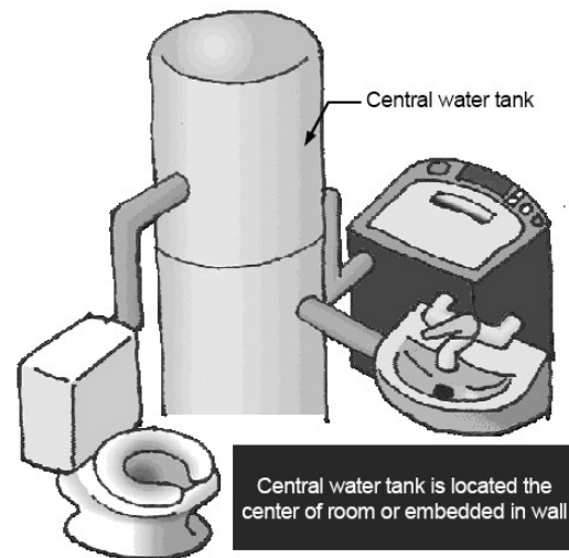
Fig. 1. Eco-friendly home grey water recycling system [13].
