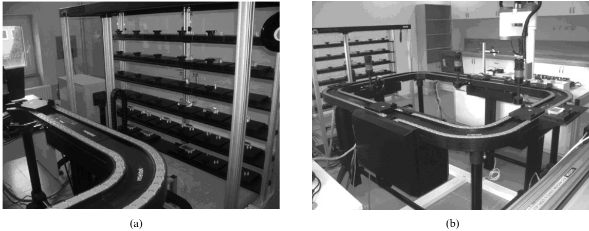
Fig. 5. Storage and material handling devices of CIM. (a) Automatic Storage and Retrieval System (AS/RS). (b) Closed loop conveyor.
