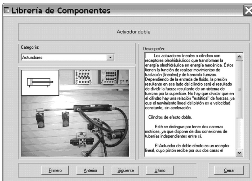
Fig. 9. Description of the hydraulic actuators in the help library. Top: Name of the element selected in the pull-down menu. Left: Picture and schematic symbol. Right: Description and principle of operation of the element.
