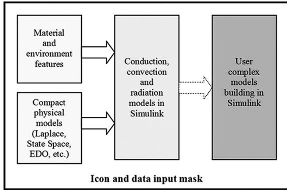
Fig. 1. Structure of heat transfer library.
